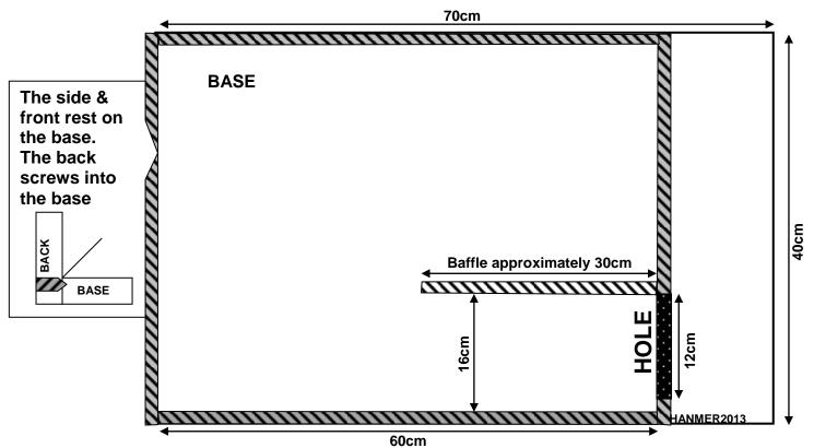
Use 18mm exterior quality ply (or something similar); paint outside only, with water based fence type paint. You can waterproof the roof lid more, with a coat of exterior gloss paint or cover with roofing felt.
